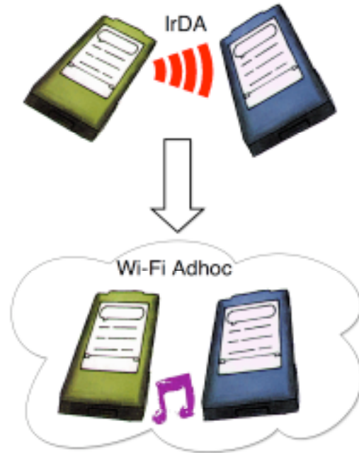
Fig. 3. Sequential Proximal Interaction: IrDA used to bootstrap an ad-hoc Wi-Fi network
